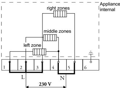
You can use the bridges provided on the connecting block to make the required interconnections as indicated in the preceding illustrations. How to install the bridges is indicated in the junction box cover and in the illustration below. The bridges should not be placed immediately on top of the connecting wires, but between the screw-head and the clamp around the connecting wire.
