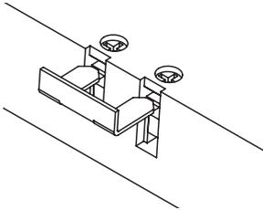
Secure the cable with the strain relief and close the cover.
