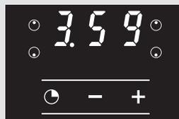
**NB:** Always switch the zone on first and then the countdown timer. The timer can be set for a maximum of 4 hours. If a zone is not switched on it cannot be linked to the timer. You can alter the preset time whenever you so require. At the end of the set time you will hear a bleep. You can switch this bleep off using the timer button. The bleep will otherwise stop automatically after 30 minutes.
