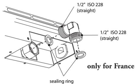
Fit the elbow supplied on the appliance's gas connection.
