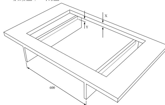
fitted-unit dimensions for HG76/77/96/97..MX/MT and HG96..SX/ST in 60 cm corpus
