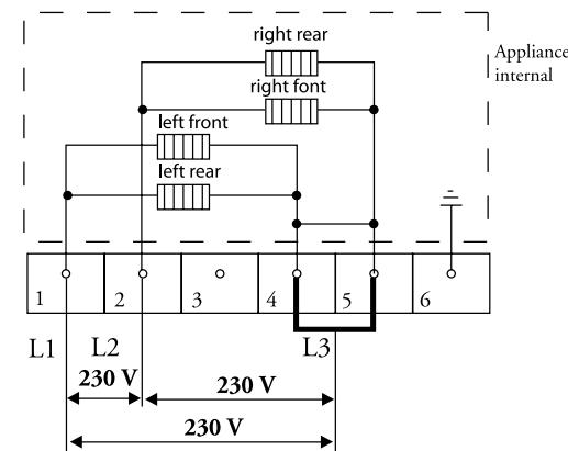
You can use the bridges provided on the connecting block to make the required interconnections as indicated in the preceding illustrations. How to install the bridges is indicated in the junction box cover and in the illustration below. The bridges should not be placed immediately on top of the connecting wires, but between the screw-head and the clamp around the connecting wire.
