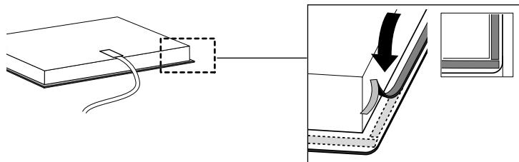
Turn the hob over and allow the appliance to sink into the opening.
