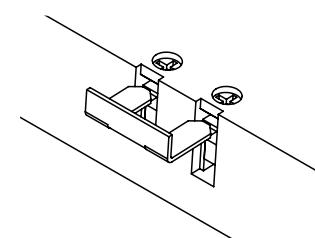
Secure the cable with the strain relief and close the cover.
