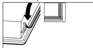
Turn the hob over and allow the appliance to sink into the opening.
