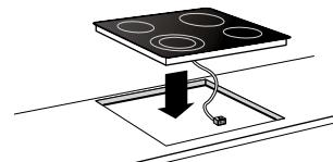
Secure the hob using the fasteners supplied.
