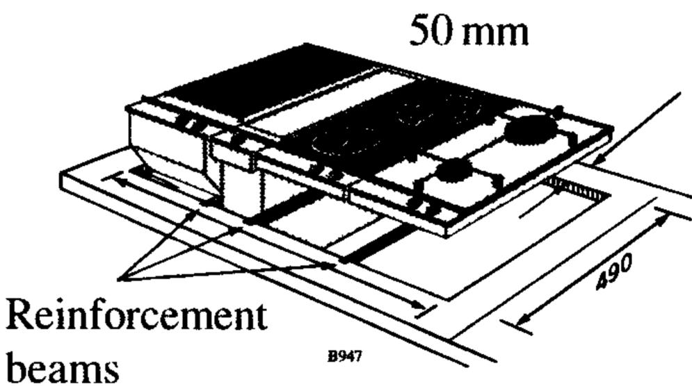
It is not necessary to attach the reinforcement beam to the table surface, as it is held in place by a specially designed moulding, which is incorporated in the hob units flanges.
