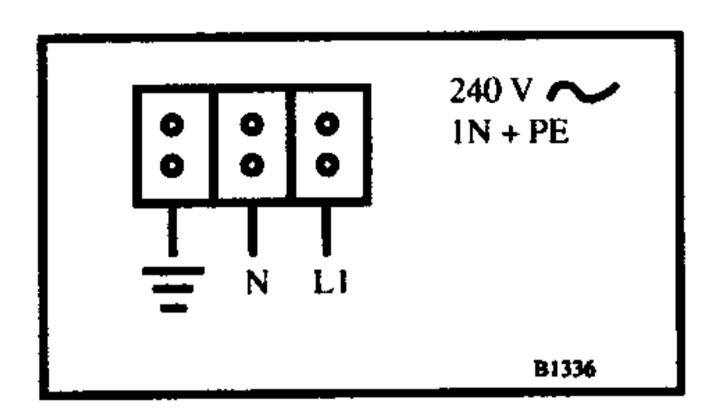
The Dropinett must be connected via an external switch with a contact gap of min. 3 mm (the main switch may be used)
