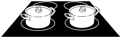
Fig. 6: Zones positioned adjacent to one another can be simultaneously set to level 12
