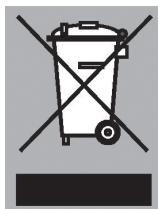
To designate the requirement for separate collection of household electrical appliances, the symbol of a dustbin with a cross through it is applied to the product. This means that the appliance may not be included with normal domestic refuse at the end of its service life. The appliance must be taken to a special municipal centre for separated waste collection or to a dealer providing this service.
