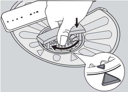
8. Put the filter (A) into position in filter (B).
