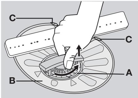
2. Filter (A) has two parts. To disassemble the filter, pull them apart.
