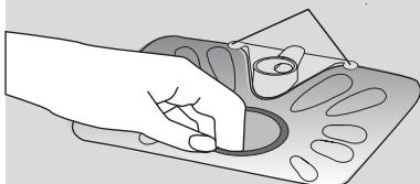
8. Place the coarse filter (**A**) in the microfilter (**B**) and press together.
