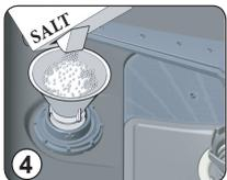
This machine is equipped with a water softener. To use the water softener, fill the dishwasher with salt.
