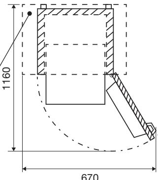
Make sure there is sufficient space around the appliance so a good ventilation and air flow around the appliance is possible.
