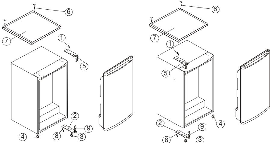
1. Remove the cover plates and screws (6) holding the top panel (7) to the unit.
