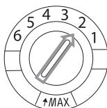
The rinse agent reservoir has 6 settings. To begin with, set the reservoir to setting 2. If this still causes spotting on the dishes, you can increase the amount of rinse agent added by turning the selector knob on the reservoir to setting 3. If there is still no improvement, turn the selector knob to a higher setting. Repeat this action until the dishes are streak-free when they emerge from the dishwasher.
