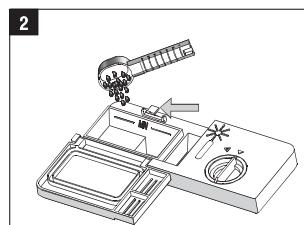
1. Press the release catch if the lid is closed. The lid will spring open.
