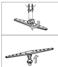
It is essential that you clean the spray arms on a regular basis. In the longer term, waste can block the nozzles and the bearings in the spray arms. Clean the spray arms as follows:
