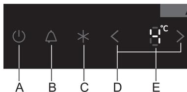
**Switching the appliance on:** Switch on the appliance by briefly pressing the key **A**.
