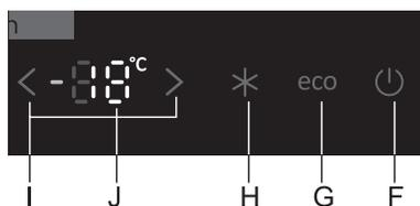
**Switching off the appliance:** To switch off the appliance, press and hold (for three seconds) the key **F** (caution: appliance will remain powered, i.e. there will still be electric current in the appliance).
