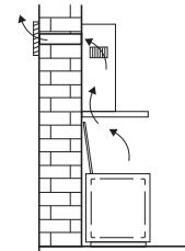
2. Recirculation hood. When the hood is connected as a recirculation hood, the grease particles and odour in the extracted vapours are filtered.
