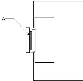
The "door open" indicator (A) at the end of the freezer door indicates if the door is shut properly.
