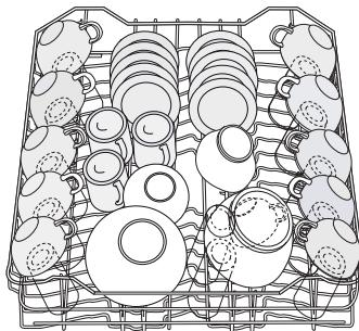
Glasses with long stems can be placed upside down in the cup racks.
