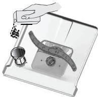
This machine is equipped with a water softener. To use the water softener, fill the dishwasher with salt.
