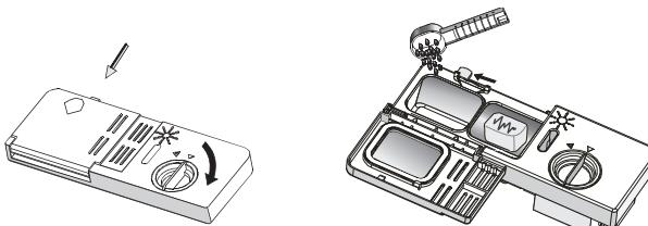
1. Press the release catch if the lid is closed. The lid will spring open.
