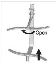
It is essential that you clean the spray arms on a regular basis. In the longer term, waste can block the nozzles and the bearings in the spray arms. Clean the spray arms as follows:
