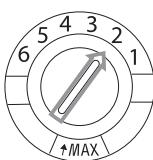
The rinse agent reservoir has 6 settings. To begin with, set the reservoir to setting 2. If this still causes spotting on the dishes and the dishes do not dry well, you can increase the amount of rinse agent added by turning the selector knob on the reservoir to setting 3. If there is still no improvement, turn the selector knob to a higher setting. Repeat this action until the dishes are streak-free when they emerge from the dishwasher.
