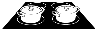
Fig. 5: Zones positioned adjacent to one another can be simultaneously set to level 12
