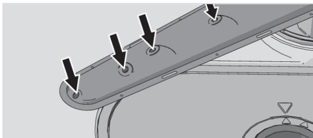
To facilitate cleaning you can remove the spray arms. Remember to fit them firmly back into place afterwards.
