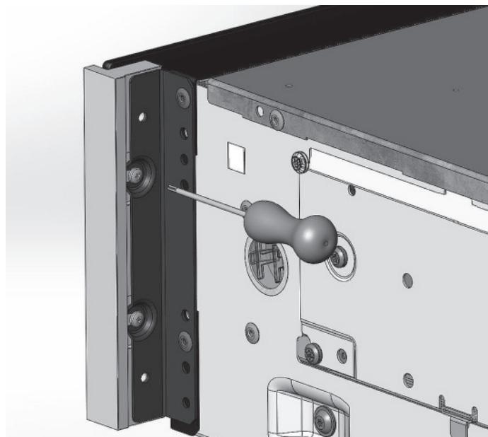
The front can be adjusted by a few millimetres for alignment with other appliances. Use the Allen key at the bottom of the appliance for this.
