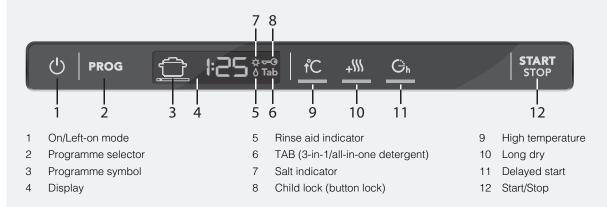
The panel is fitted with touch buttons with audible feedback (see the chapter Settings).
