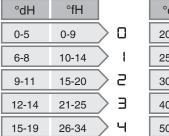
Do not forget to put salt in the salt compartment after you have set the water softener to 1 - 9.
