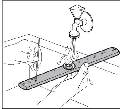
4. To engage again the spray arm to the basket, press the spray arm upwards in the direction indicated by the lower arrow and simultaneously turn it counterclockwise until it locks into place.
