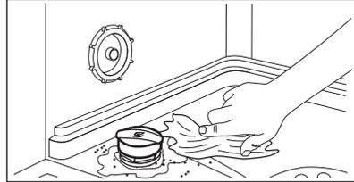
6. Turn the cap of the salt container clockwise to close the salt container.
