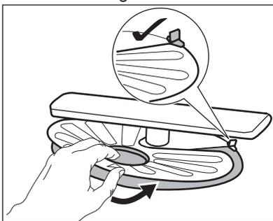
7. Reassemble the filters (B) and (C).
