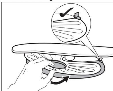
7. Reassemble the filters (B) and (C).
