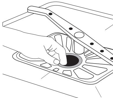
7. Put the flat filter back in the base of the washing compartment and ensure that it fits perfectly.
