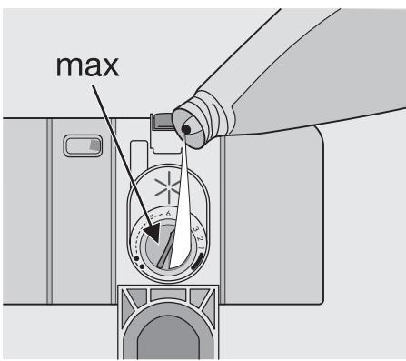
The dispenser holds about 110 ml of rinse aid, which is sufficient for between 16 and 40 washing cycles, depending upon the dosage setting.
