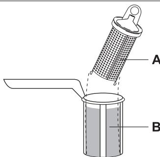
3. Turn the handle about 1/4 a turn anti-clockwise and remove the filter system
