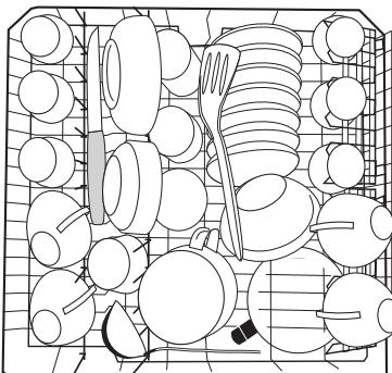
Glasses with long stems can be placed upside down in the cup racks. For taller items the cup racks can be folded upwards.
