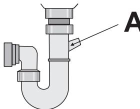
**i** Our appliances are supplied with a security device to protect against the return of dirty water back into the machine. If the spigot of your sink has a "no return valve" incorporated this can prevent the correct draining of your dishwasher. We therefore advise you to remove it.
