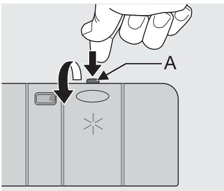
2. Add the rinse aid in the container. The maximum level for filling is indicated by "max".
