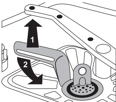
4. Take hold of the coarse filter (**A**) by the handle with the hole and remove from the microfilter (**B**).
