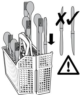
If the handles protrude from the bottom of the basket, obstructing the lower spray arm, load the cutlery with the handles facing upwards. Mix spoons with other cutlery to prevent them from sticking together.
