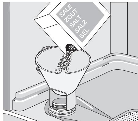
4. Replace the cap making sure that there is no trace of salt on the screw thread or on the gasket.
