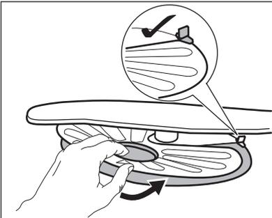
7. Reassemble the filters (B) and (C).
