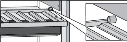
The shelf can be partly extended (pulled out from the appliance). The blocks on the cell protect the shelf from being fully extended and pulled out, which could result in the shelf falling from the appliance.
