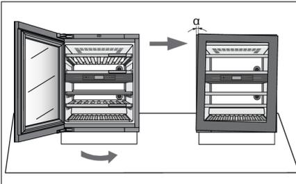
15. If the door is not aligned with the housing (the angle  $\alpha$  is not  $0^\circ$ ),
