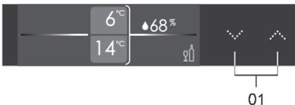
After selecting zone A or zone B, you can change setpoint temperature by pressing on 'Up/down' key (01).
