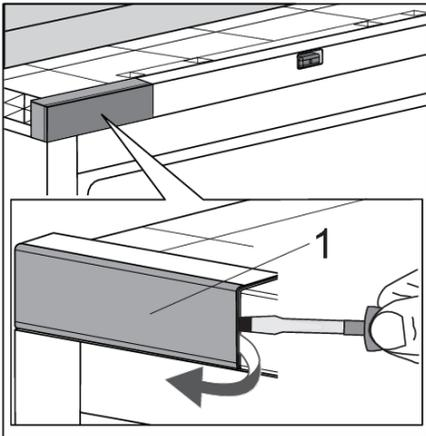
3. Open the appliance door. Carefully remove the upper hinge housing cover (1) with the help of a flat-head screwdriver. Set it aside, as you will need it later on. In case you have changed door opening direction, start in the top right-hand corner.
