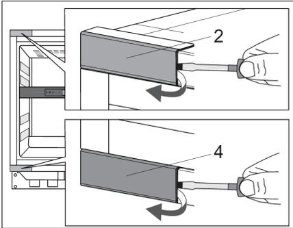
4. Carefully remove the upper (2) and bottom (4) hinge housing covers with the help of a flat-head screwdriver. Set them aside, as you will need them later on.
