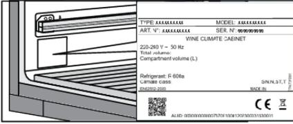
Place the appliance in a dry and well aired room. The permitted ambient temperature range for the appliance depends on the appliance's climate class, which is shown on the type plate.
