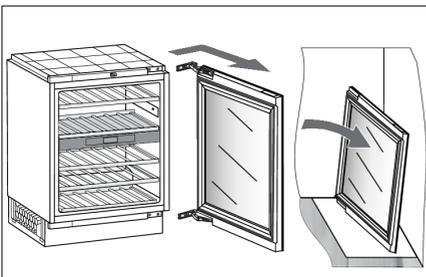
3. Remove the door, complete with the hinges, by moving it in the direction indicated by the arrow. Carefully place the door on the surface prepared for this purpose.
