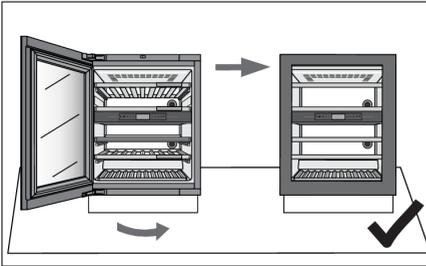
14. Close the door and make sure it is aligned with the housing. The housing side and the edge of the door should be parallel.
