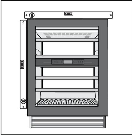
2. The appliance must be aligned horizontally and vertically, otherwise it may deform and it will not be possible to close the door properly.
