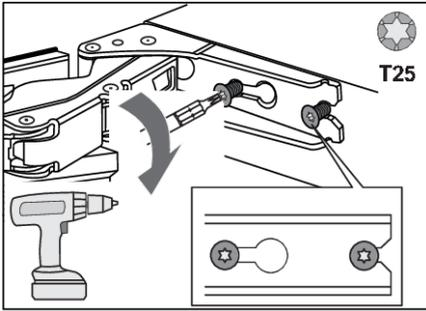
13. Tighten the screws. The screws should be tightened to a torque of 6.2 Nm.
