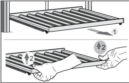
To remove a shelf from the appliance, fully extend the telescopic rails (1), and then vertically lift the shelf (2) to remove it from the rails. When removing the shelf, you can experience some resistance because of the fixation with the pin on the front side. Take care not to damage the door gasket.
