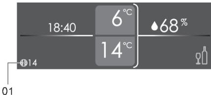
When Charcoal filter countdown timer is = 0 then Charcoal filter icon (01) is blinking normal in Status Screen.
