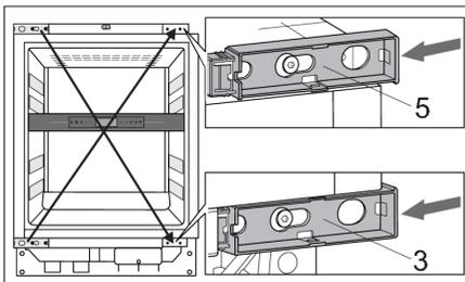
9. Take the already removed hinge housings (3, 5) and slide them into place on the diagonal position.
