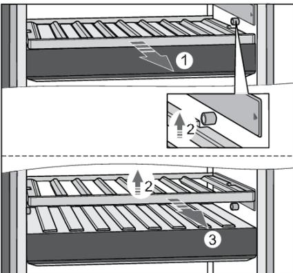
To remove a shelf from the appliance, partly pull it towards you (1) until the two grooves on the shelf and the two blocks (left, right) on the cell are aligned. Then, lift the shelf (2) and pull it out from the appliance (3). Take care not to damage the door gasket.
