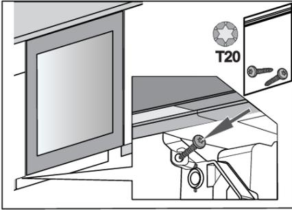
7. Attach the appliance to the adjacent kitchen element at the bottom, on the opposite side of the hinge.
