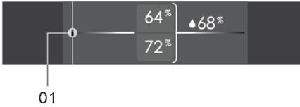
Humidity cannot be controlled, only monitored. Top value is for ZONE A and bottom value is for ZONE B. On the right side is the average humidity. The information tab (01) gives extra information about how humidity is related to wine.
