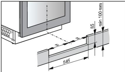
15. Prepare the plinth board. The cut-out in the plinth board for the ventilation grille must be centred with the appliance. This is the only way to ensure correct operation of the appliance.
