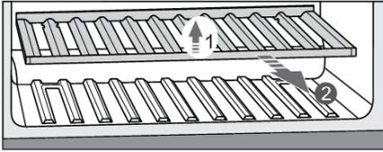
The wooden bottom bottle rack is intended for storing the bottles in the compressor area. This area is suitable for storing bottles you wish to keep for a longer period of time, especially for ageing without excessive vibration and unnecessary movement. To remove bottom rack from the appliance, lift it (1) and take it out (2). Take care not to damage the door gasket.
