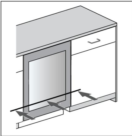
5. Push the appliance into the niche until the front surface of the door is aligned with kitchen cabinet door.
