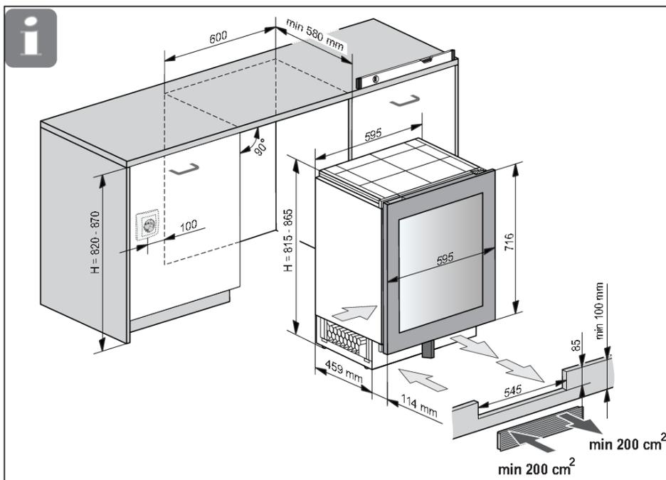
Ventilation of the appliance takes place through the slots in the base. These must not be covered. In addition, dust must be regularly cleaned from the slots.
