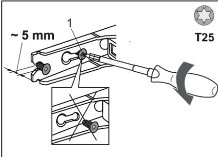
2. Partly (by no more than 5 mm) undo the hinge screws (1) at the top and bottom. Do not completely undo the screws. This way, the door will remain in contact with the housing.
