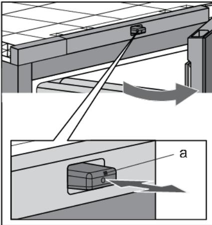
The mechanism's push pin (a) moves forward, and the door opens by approximately 6 cm. Then, you can fully open the door. If you do not open the door completely, it will automatically close. The soft-close mechanism gently closes the door.
