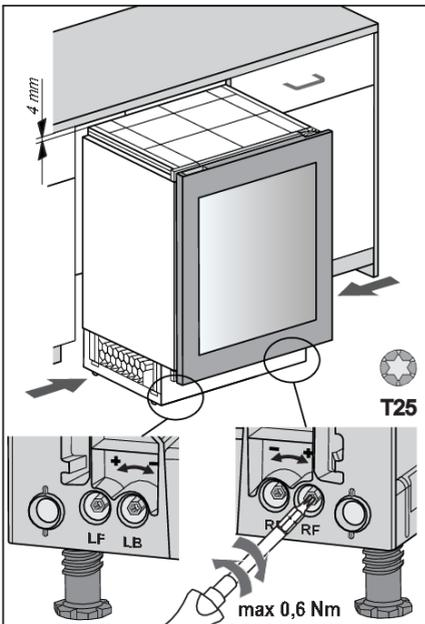
1. Before pushing the appliance into the niche, set the height of the appliance to 4 mm less than the opening.
