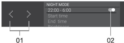
By pressing on 'Menu left/right' key (01), you can (de)activate toggle switch (02) to (de)activate a setting.
