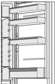
The height of the door compartments is adjustable. Lift the compartment out of the groove and fit it in the required position. Each compartment can carry a maximum weight of 5 kg. The bottom door compartment is suitable for bottles.
