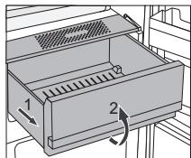
To remove a drawer, pull out the drawer as far as it will go (1). Then, lift the front part (2) and pull it out completely.
