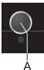
**Switching the appliance on:** Press the A key and hold it for 3 seconds.
