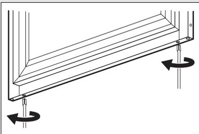
With the door open, loosen the two screws situated in the lower part without unscrewing them completely.
