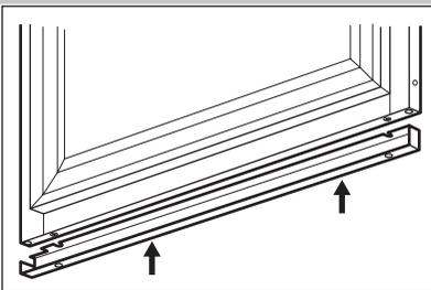
Position the steel compensator as indicated in the figure and insert the upper part under the head of the screws.
