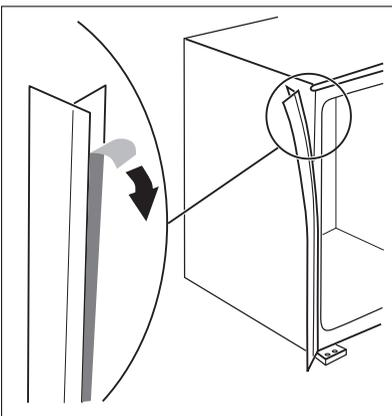
Apply the adhesive sealing strip to the appliance as shown in figure.
