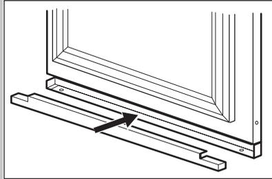
Insert the steel carter inside the compensator as indicated in the figure.
