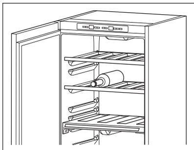
Remove the shelf and insert it between the two guides.
