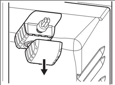
At the same time, free the middle hook and slide off the cover in the direction of the arrows.
