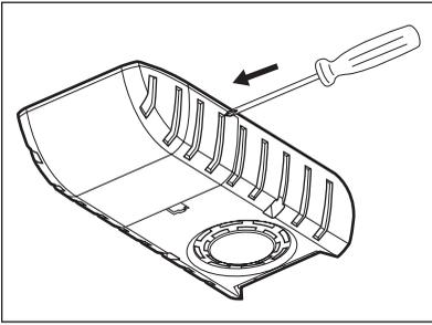
Remove the lamp cover by pressing it inwards with a tool (e.g. screwdriver) to free the rear side hookings.
