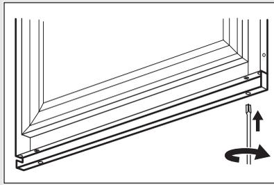
Align the compensator with the steel door panel and tighten the screws.
