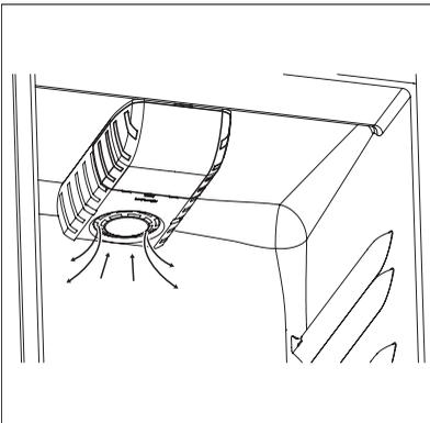
The refrigerator compartment has a special AIRLIGHT fan which is automatically activated in function of the appliance thermostat setting and ambient conditions.
