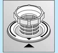
Screw in filter system **NOTE MARK!**
