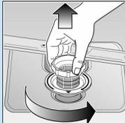
Rotate filter cylinder, remove filter system ...
