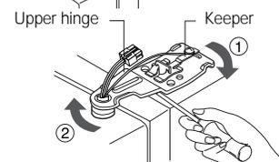
3) Remove the refrigerator compartment door by lifting it up.
