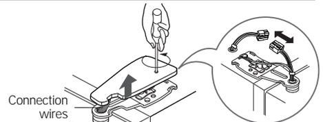
2) Remove keeper by rotating it clockwise (ⓐ) and then remove the upper hinge by lifting it up (ⓑ).
