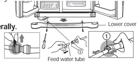
**Remove lower cover and then feed water tube**
