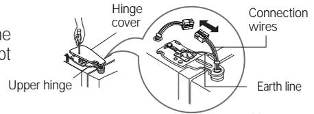
2) Remove the keeper by rotating it counter clockwise (ⓐ) and then lifting the upper hinge up (ⓑ).
