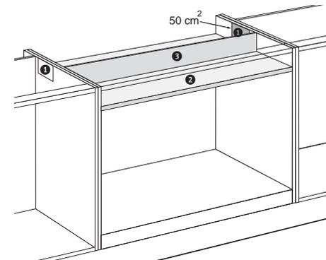
Fit a protective plate between the oven and the hob. The plate should be at least 10 mm thick and heat-resistant (85 °C). The space between the underside of the hob and the protective plate must be at least 50 mm.
