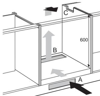
Recess height minimum 600 mm. Ventilation is via plinth and rear of oven. Where there is a oven, a gap of at least 560 x 6 mm should be made at the front. Cut out ventilation openings "A" + "B" (100 cm<sup>2</sup>). Make an opening in the side wall "C" of the kitchen cupboard for leading the connection cable through. The hob may only be combined with ATAG ovens, not with combi-microwave ovens.
