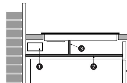
To protect the air flow, fit a protective panel - of the same material as the protective plate - between the protective plate and the hob. Ventilation is via the adjoining cupboards.
