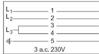
If you want to make a fixed connection, make sure that a multi-polar switch with a contact separation of at least 3 mm is fitted in the supply line.
