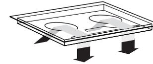
The electronics in the appliance require cooling. The ventilation openings are located on the underside of the appliance. It must be possible for cool air to be drawn in through these openings. The appliance is fitted with outlet openings at the front and bottom. The kitchen unit will require a few modifications to allow optimum cooling of the hob.
