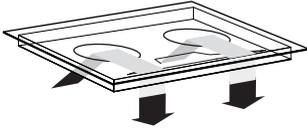
The electronics in the appliance require cooling. The ventilation openings are located on the underside of the appliance. It must be possible for cool air to be drawn in through these openings. The appliance is fitted with outlet openings at the front.
