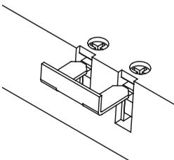
You can use the bridges provided on the connecting block to make the required interconnections as indicated in the preceding illustrations. How to install the bridges is indicated in the junction box cover and in the illustration below. The bridges should not be placed immediately on top of the connecting wires, but between the screw-head and the clamp around the connecting wire. Secure the cable with the strain relief and close the cover.
