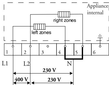
Install a connecting bridge between the connection points 4-5. Your groups must be fused with at least 16 A (2x). The connecting power cable must have a minimum core cross section of 2,5 mm<sup>2</sup>.
