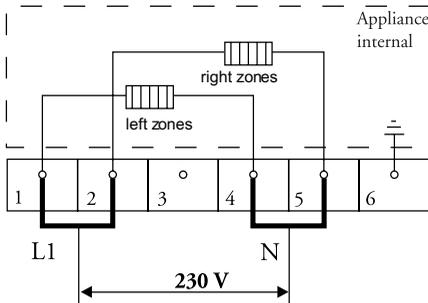
Install connecting bridges between connection points 1-2 and 4-5. Your group must be protected by a fuse of at least 32 A. The connecting power cable must have a minimum core cross section of 6 mm<sup>2</sup>.
