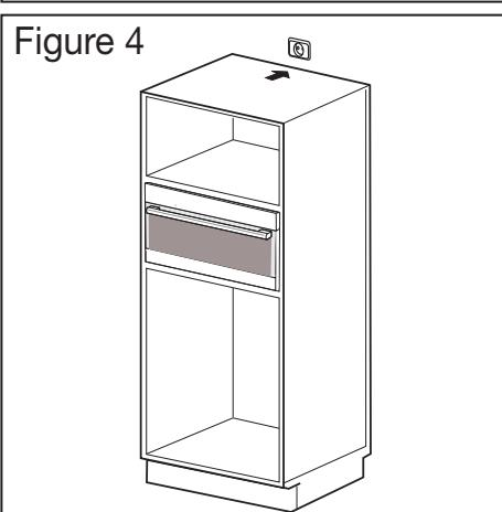
Fig1. Slide the oven partly into the recess. Lead the connection cable to the power source.
