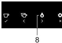
3. Press the 'Hot water' touch key (8). Hot water is dispensed; the display shows "HOT WATER". Once the programmed amount of hot water is dispensed, dispensing stops automatically. For a few seconds the display shows "PREPARATION RUNNING PLEASE WAIT". After that the appliance is ready to make coffee again and the last selected coffee setting appears on the display.
