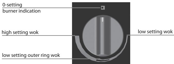
Press the control knob in and turn it anti-clockwise.
