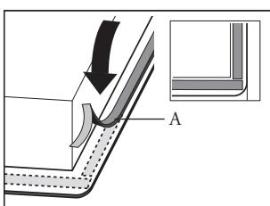
Remove the protective foil of the sealing strip (A) and attach the sealing strip in the groove of the aluminium profiles or the edge of the glass plate. Do not attach the sealing strip through the corner. Instead, cut 4 pieces that fit tightly together in the corners.
