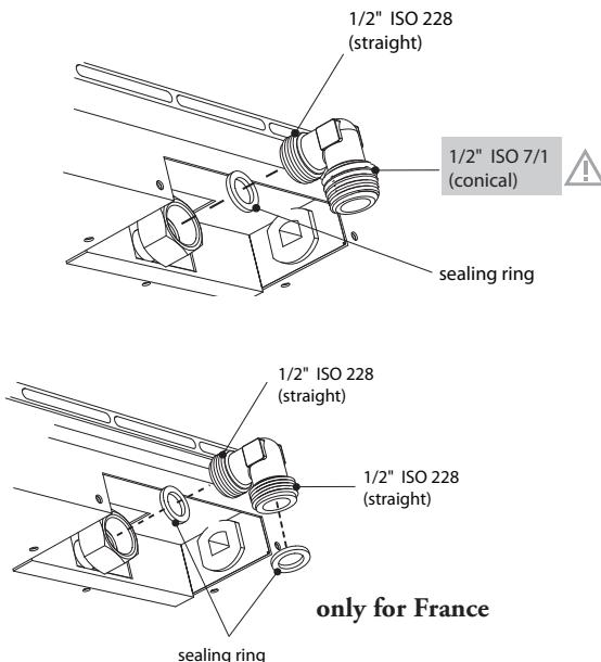
Fit the elbow supplied on the appliance's gas connection.
