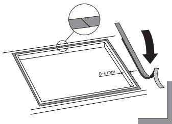
Remove the protective foil from the sealing tape and apply the tape around the cut-out in the worktop. Start at the rear side of the appliance and tape the sealing strip along the corners. Make sure that the ends of the sealing strip fit tightly together.
