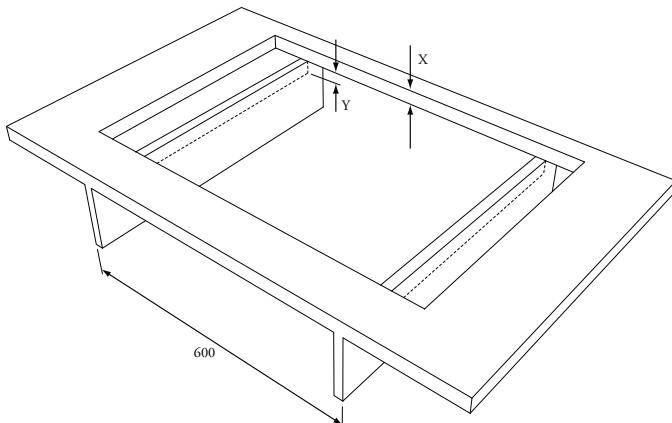
fitted-unit dimensions for HG76/77/96/97..MB and HG96..SB in 60 cm corpus
