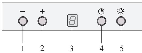
1. Reduce extractor capacity and switch fan off
