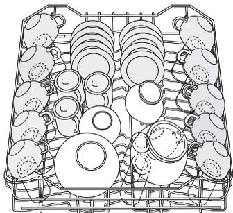
Glasses with long stems can be placed upside down in the cup racks. For taller items, the cup racks can be folded upwards.
