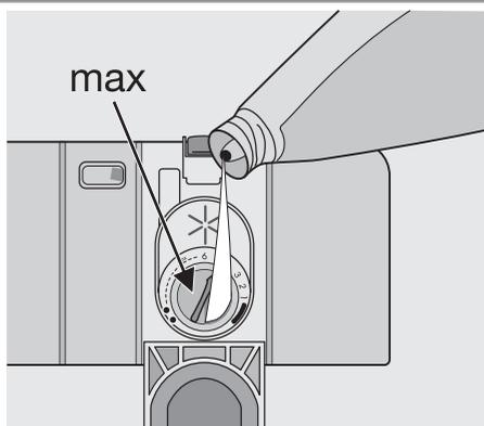
The dispenser holds about 110 ml of rinse aid, which is sufficient for between 16 and 40 washing cycles, depending upon the dosage setting.
