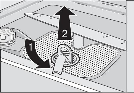
4. Take hold of the coarse filter (A) by the handle with the hole and remove from the microfilter (B).
