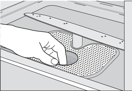
7. Put the flat filter back in the base of the washing compartment and ensure that it fits perfectly.
