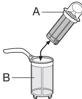
3. Turn the handle about 1/4 a turn anti-clockwise and remove the filter system
