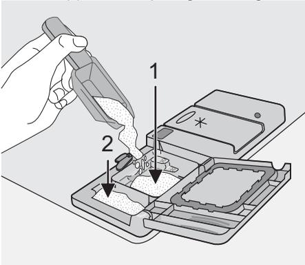
3. All programmes with prewash need an additional detergent dose (5/10 g) that must be placed in the prewash detergent chamber (2). This detergent will be used during the prewash phase. When using detergent tablets; place the tablet in compartment (1)
