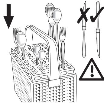
If the handles protrude from the bottom of the basket, obstructing the lower spray arm, load the cutlery with the handles facing upwards. Mix spoons with other cutlery to prevent them from sticking together.
