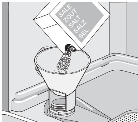
4. Replace the cap making sure that there is no trace of salt on the screw thread or on the gasket.
