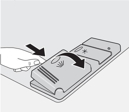
2. Fill the detergent dispenser (1) with detergent. The marking indicates the dosing levels:
