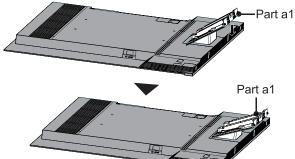
4. Secure Part a1 with 4 screws (M5×12) onto the back cover of the TV.
