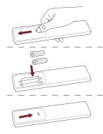
1. Slide the back cover to open the battery compartment of the remote control.
